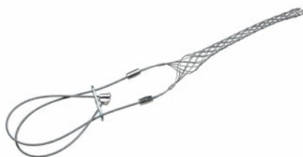
FC52LB: Bus Drop, Closed Mesh, Locking Bale, Cable Diameter 0.53 - 0.73 inches, Bale Length 15-in, Mesh Length 6.5-in, Break Strength 1100 lbs.
