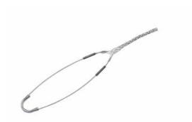
FC70: Bus Drop, Closed Mesh, Single Eye, Cable Diameter 0.70 - 0.85 inches, Bale Length 9-in, Mesh Length 8.5-in, Break Strength 1900 lbs.
