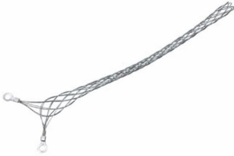
FC70GL: Extra-Hard Use, Closed Mesh, Cable Diameter 0.70 - 0.85 inches, Mesh Length 8.5-in
