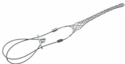
FC70LB: Bus Drop, Closed Mesh, Locking Bale, Cable Diameter 0.70 - 0.85 inches, Bale Length 16-in, Mesh Length 8.5-in, Break Strength 1900 lbs.
