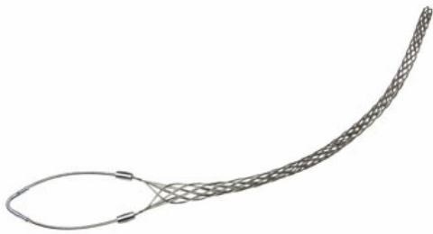
FCHL100U: Standard Duty, Closed Mesh, Single-Eye Grip, Cable Diameter 1.00 - 1.24 inches, Bale Length 10-in, Mesh Length 29-in, Break Strength 4720 lbs.
