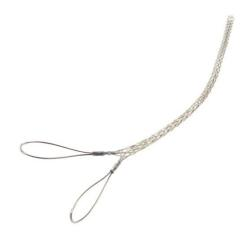
FCHL100UU: Heavy-Duty, Closed Mesh, Double-Eye, Cable Diameter 1.00 - 1.24 inches, Bale Length 10-in, Mesh Length 29-in, Break Strength 4720 lbs.
