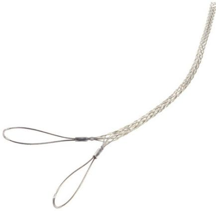
FCHL100UU: Heavy-Duty, Closed Mesh, Double-Eye, Cable Diameter 1.00 - 1.24 inches, Bale Length 10-in, Mesh Length 29-in, Break Strength 4720 lbs.
