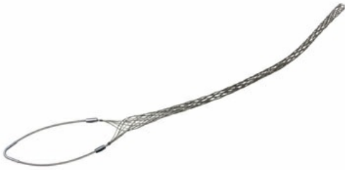
FCHL150U: Standard Duty, Closed Mesh, Single-Eye Grip, Cable Diameter 1.50 - 1.99 inches, Bale Length 10-in, Mesh Length 35-in, Break Strength 4720 lbs.
