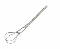
FCSD52LB: Service Drop, Closed Mesh, Locking Bale, Cable Diameter 0.53 - 0.73 inches, Bale Length 14-in, Mesh Length 8-in, Break Strength 790 lbs.
