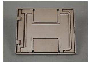
Flangeless cover for use in tile installation. Die-cast aluminum assembly. Insert in lid allows for tile cutouts to match finished floor. NOTE: Add suffix "TR" to the end of the part number to indicate tamper-resistant cover assembly. Tamper-resistant versions are secured with a single tamper-resistant screw.
