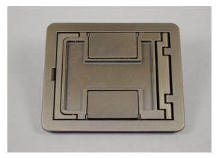
Flanged cover for use in tile or carpet installation. Die-cast aluminum assembly. Insert in lid allows for carpet or tile cutouts to match finished floor. NOTE: Add suffix "TR" to the end of the part number to indicate tamper-resistant cover assembly. Tamper-resistant versions are secured with a single tamper-resistant screw. "NA" indicates North American made and complies with the Buy American Act, NAFTA, and ARRA requirements.
