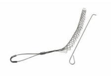
FR0500F: Standard Duty, Split Rod, Offset Eye, Cable Diameter 0.50 - 0.61 inches, Bale Length 4-in, Mesh Length 11-in
