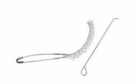
FR050U: Standard Duty, Split Rod, Single Eye, Cable Diameter 0.50 - 0.61 inches, Bale Length 7-in, Mesh Length 11-in, Break Strength 770 lbs.
