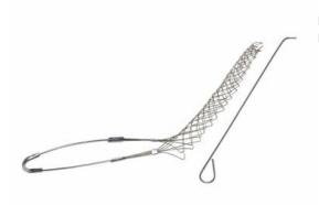
FR062U: Standard Duty, Split Rod, Single Eye, Cable Diameter 0.62 - 0.74 inches, Bale Length 8-in, Mesh Length 11-in, Break Strength 960 lbs.
