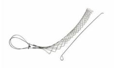
FR100LB: Standard Duty, Split Rod, Locking Bale (Universal Eye), Cable Diameter 1.00 - 1.24 inches, Bale Length 14-in, Mesh Length 13-in, Break Strength 1920 lbs.
