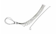
FR125LB: Standard Duty, Split Rod, Locking Bale (Universal Eye), Cable Diameter 1.25 - 1.49 inches, Bale Length 14-in, Mesh Length 15-in, Break Strength 1920 lbs.
