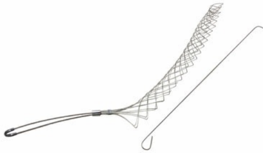
FR125U: Standard Duty, Split Rod, Single Eye, Cable Diameter 1.25 - 1.49 inches, Bale Length 10-in, Mesh Length 16-in, Break Strength 1680 lbs.
