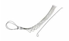
FR150LB: Standard Duty, Split Rod, Locking Bale (Universal Eye), Cable Diameter 1.50 - 1.74 inches, Bale Length 14-in, Mesh Length 16-in, Break Strength 1920 lbs.
