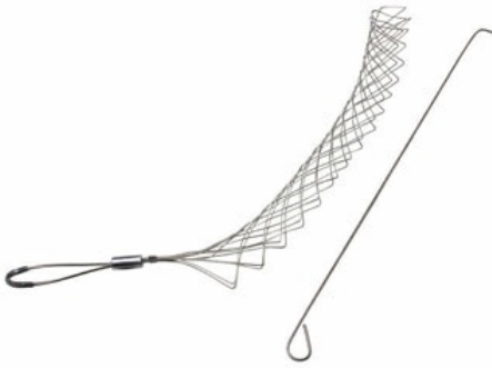
FR1500F: Standard Duty, Split Rod, Offset Eye, Cable Diameter 1.50 - 1.74 inches, Bale Length 5-in, Mesh Length 18-in
