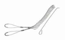
FR200UU: Standard Duty, Split Rod, Double-Eye, Cable Diameter 2.00 - 2.49 inches, Bale Length 6-in, Mesh Length 22-in, Break Strength 3750 lbs.
