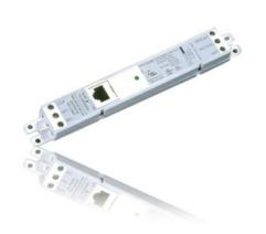
The FS-PP Fixture Power Pack provides 24 VDC operating voltage to the FS Low Voltage Sensor series via the RJ45 connector built onto each sensor. The incorporated Form-C Relay, Normally Open (N/O)/Normally Closed (N/C), can control line or low voltage loads.
