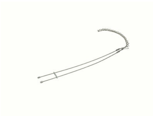
FS050LB: Standard Duty, Split Lace, Locking Bale (Universal Eye), Cable Diameter 0.50 - 0.61 inches, Bale Length 18-in, Mesh Length 11-in, Break Strength 770 lbs.
