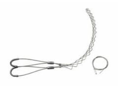
FS050UU: Standard Duty, Split Lace, Double-Eye, Cable Diameter 0.50 - 0.61 inches, Bale Length 4-in, Mesh Length 11-in, Break Strength 770 lbs.
