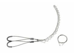
FS062UU: Standard Duty, Split Lace, Double-Eye, Cable Diameter 0.62 - 0.74 inches, Bale Length 4-in, Mesh Length 11-in, Break Strength 1150 lbs.
