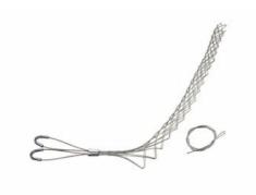
FS100UU: Standard Duty, Split Lace, Double-Eye, Cable Diameter 1.00 - 1.24 inches, Bale Length 5-in, Mesh Length 15-in, Break Strength 1920 lbs.
