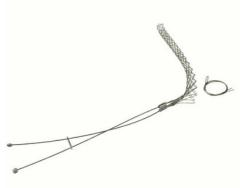
FS125LB: Standard Duty, Split Lace, Locking Bale (Universal Eye), Cable Diameter 1.25 - 1.49 inches, Bale Length 18-in, Mesh Length 16-in, Break Strength 1920 lbs.
