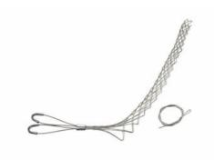
FS125UU: Standard Duty, Split Lace, Double-Eye, Cable Diameter 1.25 - 1.49 inches, Bale Length 5-in, Mesh Length 16-in, Break Strength 1920 lbs.
