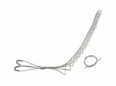
FS150UU: Standard Duty, Split Lace, Double-Eye, Cable Diameter 1.50 - 1.74 inches, Bale Length 5-in, Mesh Length 18-in, Break Strength 1920 lbs.
