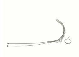
FS175LB: Standard Duty, Split Lace, Locking Bale (Universal Eye), Cable Diameter 1.75 - 1.99 inches, Bale Length 18-in, Mesh Length 20-in, Break Strength 3150 lbs.
