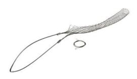
FS200U: Standard Duty, Split Lace, Single Eye, Cable Diameter 2.00 - 2.49 inches, Bale Length 16-in, Mesh Length 22-in, Break Strength 3760 lbs.
