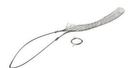
FS200U: Standard Duty, Split Lace, Single Eye, Cable Diameter 2.00 - 2.49 inches, Bale Length 16-in, Mesh Length 22-in, Break Strength 3760 lbs.
