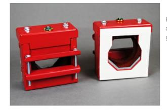
For transitioning cable through fire rated walls/floors for both new and retrofit applications. Available in red (RED), or a paintable A60 galvaneal finish (GA). UL System W-L-3264 and W-J-3137.
