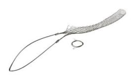
FS300U: Standard Duty, Split Lace, Single Eye, Cable Diameter 3.00 - 3.49 inches, Bale Length 21-in, Mesh Length 26-in, Break Strength 5040 lbs.
