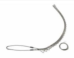
FSHL075U: Heavy-Duty, Split Lace, Single Eye, Cable Diameter 0.75 - 0.99 inches, Bale Length 10-in, Mesh Length 26-in, Break Strength 2700 lbs.
