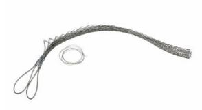
FSHL075UU: Heavy-Duty, Split Lace, Double-Eye, Cable Diameter 0.75 - 0.99 inches, Bale Length 10-in, Mesh Length 26-in, Break Strength 2700 lbs.
