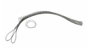
FSHL300UU: Heavy-Duty, Split Lace, Double-Eye, Cable Diameter 3.00 - 3.49 inches, Bale Length 10-in, Mesh Length 41-in, Break Strength 10080 lbs.
