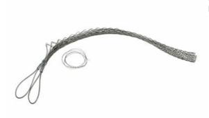
FSHL350UU: Heavy-Duty, Split Lace, Double-Eye, Cable Diameter 3.5 - 3.99 inches, Bale Length 10-in, Mesh Length 45-in, Break Strength 13120 lbs.
