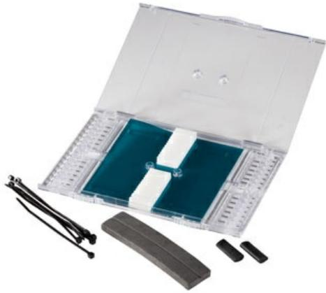
The 12-Fiber transparent fusion splice tray is ideal for fusion splicing single fiber. The see through cover and mylar insert enable easy viewing when visual fault locator (VFL) testing and verification is performed to ensure cable continuity and determine pass or failure of splicing. The hinged cover and carefully designed fiber routing enable quick and easy splicing and fiber management. The stackable design of this 7 inch tray, saves space while ensuring maximum density for the application.
