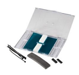
The 12-Fiber transparent fusion splice tray is ideal for fusion splicing single fiber. The see through cover and mylar insert enable easy viewing when visual fault locator (VFL) testing and verification is performed to ensure cable continuity and determine pass or failure of splicing. The hinged cover and carefully designed fiber routing enable quick and easy splicing and fiber management. The stackable design of this 7 inch tray, saves space while ensuring maximum density for the application.
