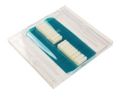
The 144-Fiber transparent fusion splice tray is ideal for fusion splicing ribbon fiber. The see through cover and mylar insert enable easy viewing when visual fault locator (VFL) testing and verification is performed to ensure cable continuity and determine pass or failure of splicing. The hinged cover and carefully designed fiber routing enable quick and easy splicing and fiber management. The stackable design of this 7 inch tray, saves space while ensuring maximum density for the application.
