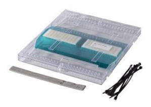
The 48-Fiber transparent fusion splice tray is ideal for fusion splicing single fiber. The see through cover and mylar insert enable easy viewing when visual fault locator (VFL) testing and verification is performed to ensure cable continuity and determine pass or failure of splicing. The hinged cover and carefully designed fiber routing enable quick and easy splicing and fiber management. The stackable design of this 7 inch tray, saves space while ensuring maximum density for the application.
