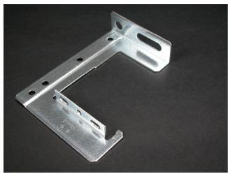
Suspends 3000 Series Raceway from structural ceilings. Designed for use with 3/8" (9.5mm) threaded rod. Hangers should be installed no more than 5" (1.5m) apart along raceway run. This C-Hanger can be mounted back-to-back for double run of 3000 Series Raceway.
