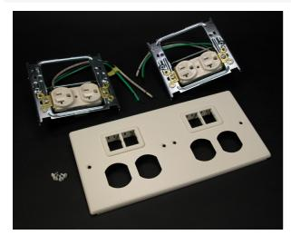
Includes two Pass and Seymour 20A Duplex Receptacles with 12" wire leads installed on bracket. Includes mini adapter that accepts two Ortronics TracJack inserts. NOTE: Certified to Canadian Safety Standards for sale in Canada. When ordering these products, change the "V" color prefix to "CV" or the "G" color prefix to "CG" to denote the Canadian versions.
