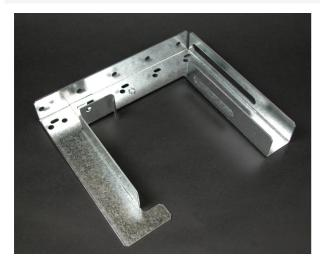
suspending 6000 or 4000 Series Raceway from structural ceiling. Designed for use with 3/8" (9.5mm) rod. Hangers should be installed no more than 5' (1.5m) apart along raceway run. Can be bolted back-to-back for dual runs of 4000, 6000 or 3008C or for combined runs with 3000 Series Raceway.
