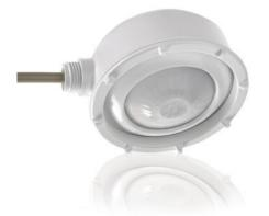
For wet locations, low bay applications, the HBL2 pattern spreads over a 48' diameter area at a height of 8'. This lens offers 360° coverage and are best suited for open area and aisleway coverage in high bay applications. This is a multi-cell, multi-tier Fresnel lens offers a high density coverage pattern.
