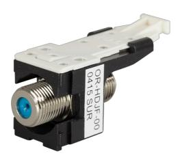
High density jack module provides a single F-connector coupler F/F with under .2dB of insertion loss at 2GHz (1/3 the loss of standard models). HDJ is a versatile single jack solution in a easy mount rear load footprint which allows a choice of up to six jacks/connectors to fit in a single gang plate, also mountable in HDJ panels.
