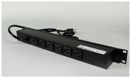
Six rear outlets, lighted switch, 15A, 6' (1.8m) cord. Receptacle center-to-center 1 1/2'' (38mm).
