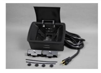
Cord-ended with black, flush cover with decorative recess. Unit comes with two 20A gasketed prewired receptacles with a 12' (3.65m) 14/3 SJT black cord. Includes adapter for Wiremold CM Series Open System communications outlets. Communication modules sold separately.
