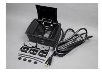
Cord-ended with black, flush cover. Unit comes with two 20A gasketed prewired receptacles with a 12' (3.65m) 14/3 SJT black cord. Includes adapter for Ortronics Series II and TracJack inserts. Communication modules sold separately.
