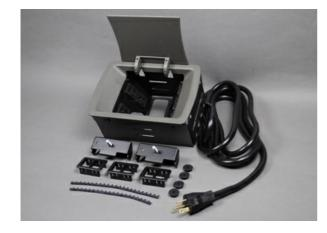
Cord-ended with gray, flush cover. Unit comes with two 20A gasketed prewired receptacles with a 12' (3.65m) 14/3 SJT black cord. Includes adapter for Ortronics Series II and TracJack inserts. Communication modules sold separately.
