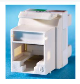
Category 6 Keystone jack, 8-position, 180 degree exit, icon compatible, T568A/B wiring. TechChoice keystone jacks and modules feature an easy-to-follow universal wiring label and support standard termination using a 110-impact tool. The keystone footprint allows for the greatest flexibility in installation scheduling because its rear insertion into the faceplate allows the technician to complete the termination before and during the construction process.
