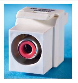
TechChoice keystone jacks and modules feature an easy-to-follow universal wiring label and support standard termination using a 110impact tool. The keystone footprint allows for the greatest flexibility in installation scheduling because its rear insertion into the faceplate allows the technician to complete the termination before and during the construction process.
