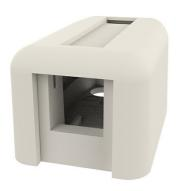
Keystone Surface Mount Boxes accept rear loading Keystone and KT2J jacks & modules and provide easy snap-on covers and snap-in label fields. Boxes are supplied with screws and double-sided adhesive tape for mounting onto almost any surface. Meet UL2043 and are suitable for installation in air handling spaces (ie plenum spaces).
